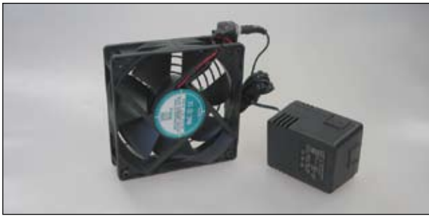
Fig. 3. A series of plug-in thermally controlled fans from Orion Fans for spot cooling are supplied with a standard plug-in transformer, giving enclosure manufacturers the ability to add them to their cabinets without rewiring.
