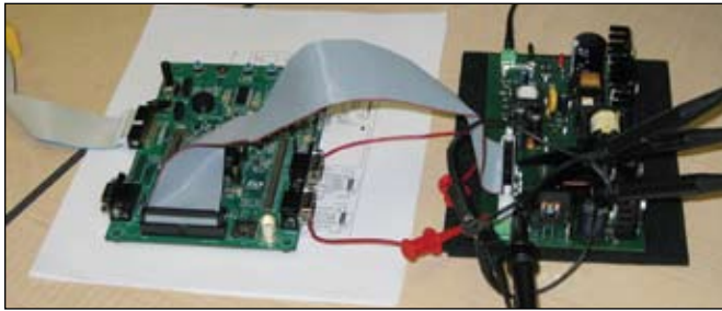
Fig. 3. The power-converter demo consists of two printed-circuit boards. The STM32 MCU board is on the left and the power-converter board is on the right.
