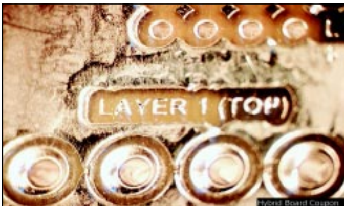
Fig. 1. Process coupon of a hybrid thick/thin copper printed wiring board (solder coated).
