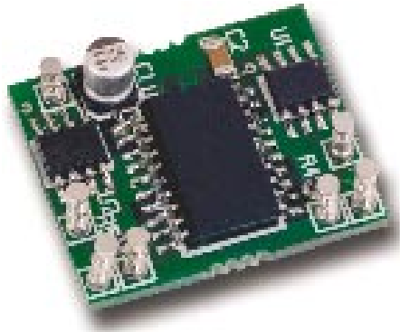
Photo 1. A 6A H-bridge control circuit in a 25 mm × 21 mm footprint.
