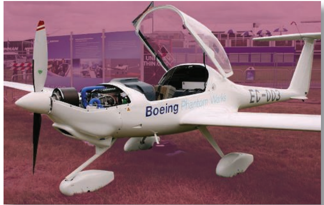
Fig. 9. Boeing Research and Technology Europe flew a fuel cell-powered modified Dimona motor-glider for 20min at its Spanish test site. achieved straight-level flight.
