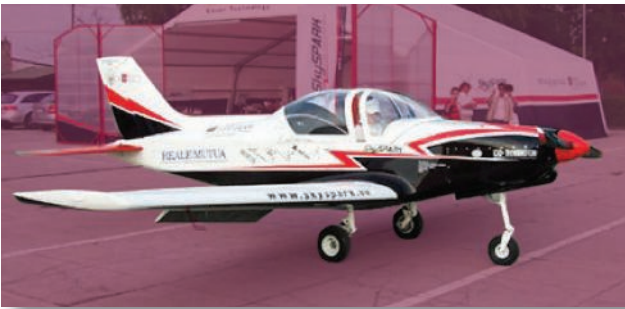
Fig. 8. SkySpark uses a hydrogen fuel cell capable of providing 65kW to power this aircraft along with a lithium polymer battery.
