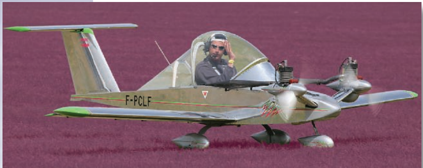
Fig. 2. Cri-Cri uses composite materials instead of metal to reduce overall weight and make room for the high-energy-density lithium batteries that provide power to four brushless electric motors - two mounted back-to-back on nose pods on each side - with counter-rotating propellers.
