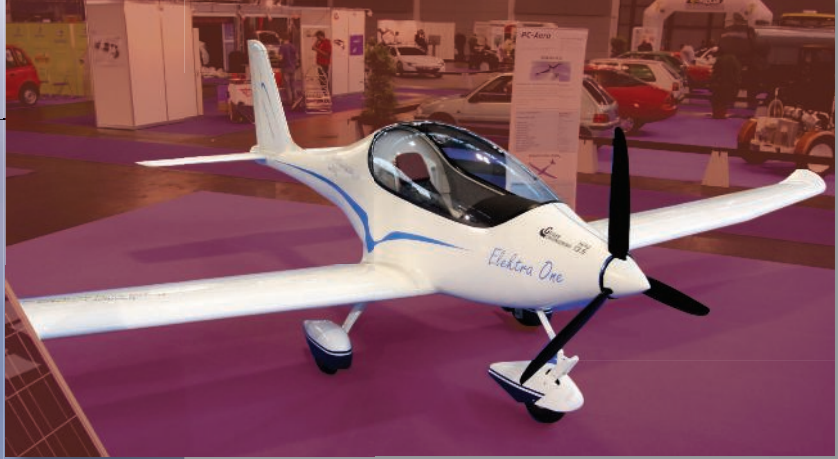
Fig. 1. Elektra One has a maximum power is 16-20 kW, and range is more than 400 km (249 miles) with a flight time of up to more than 3 hours.
