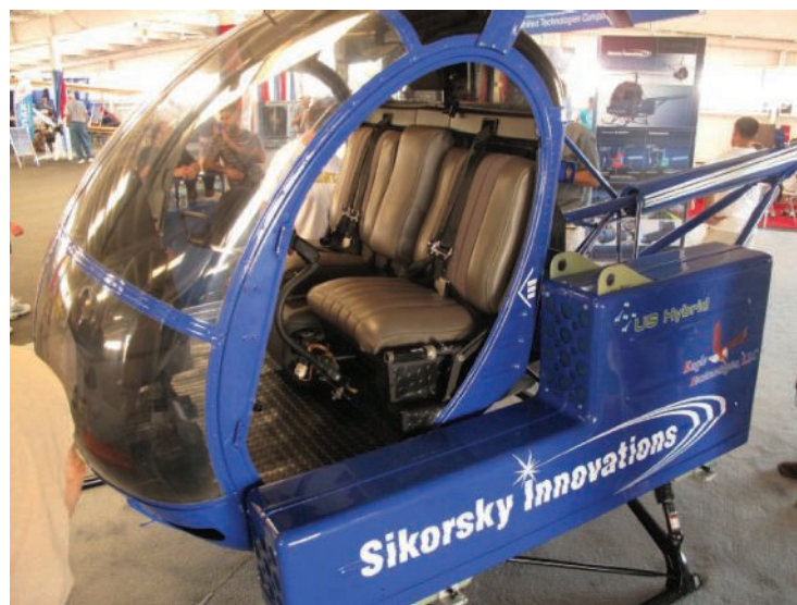
Fig. 7. Sikorsky's Project Firefly will include a 190 hp (142 kW) motor specifically tailored for use in rotorcraft. The battery pack consists of 300 cells, with an energy density of 0.13 kW per kilogram.
