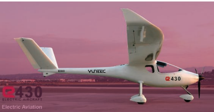
Fig. 3. The E430 uses three lithium polymer battery packs that allow it to fly for two hours in an “optimum cruise” with two people on board.
