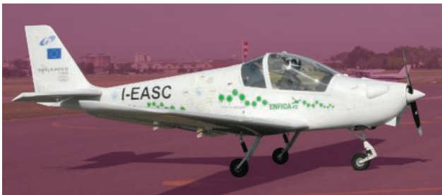
Fig. 10. Designated Rapid 200-FC, this electric aircraft was powered by an electric hybrid system consisting of a 20kW PEM fuel cell and a 20kW Li-Po battery.
